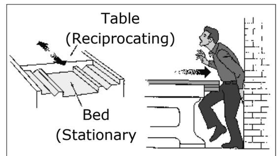
Cutting action may involve rotating, reciprocating, or transverse motion. The danger of cutting action exists at the point of operation where finger, arm, and body injuries can occur and where flying chips or scrap material can strike the head, particularly in the area of the eyes or face. Such hazards are present at the point of operation in cutting work, metal, or other materials.
